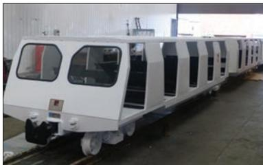
BCL Limited awarded Qualter Hall the contract for the design and manufacture of three replacement, updated Rope Hauled GMT Manriding Cars comprising 1 x 36 seat rope Hauled Anchor Car, 1 x 36 seat Leading Manrider Car and 1 x 36 seat Trailing Manrider Car.
